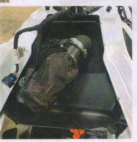
12. Install the short rubber straps in the location on the hood as shown. Install the long rubber straps on the hood as shown. Note: When tightening the longer straps, only tighten until the nyloc nut gets past the threads on the screw. Tighten so the strap can move back and forth without too much resistance.
