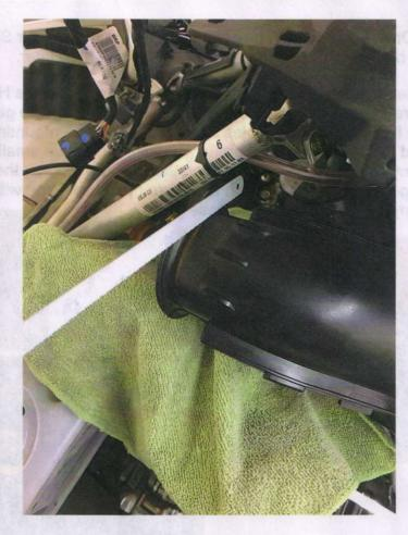
5. Once you have carefully cut off the flared end, clean up the edges with sandpaper and remove all burrs and debris. Install the hose that was included in your kit along with the hose clamp. Note: This hose is a tight fit and will go on to provide a nice fit. Work it on the intake carefully and then install the hose clamp.
