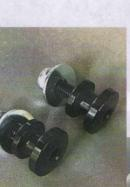
8. Locate the turned catches in your hardware kit. Install these rubber strap catches in the locations shown in the pictures below on the hood side panels. Be sure to place the flat washer and nyloc nuts on the back. Tighten.
