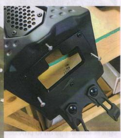
Next, you will need to prepare the inlet of the intake for the new hose. Stuff a towel or rag in the inlet of the r intake box. Place a rag or towel over the clutch and engine area to catch debris as shown. Remove the OEM rubber adapter. Mark the intake
