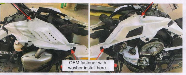
Once the hood side panels are installed, you can install the air box partition. The 6 holes are pre-drilled in the hood side panels and the air box partition. Place the partition in position and line up the holes. Install plit rivets included in your kit. Be sure you use a clamp to hold the pieces together before you pull the rivets. Route the air intake tube up through the hole in the air box partition as shown.
