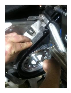
While holding composite belt guard in place, insert lower Carbon Fiber belt guard / speed sensor plate into position, and install retaining bolts.
