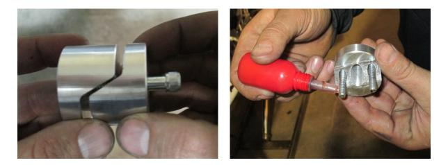
Step 8: Reinstall the 1/4 - 20 bolts into lower pulley retainer finger tight. Install retainer assembly into lower driveshaft.
