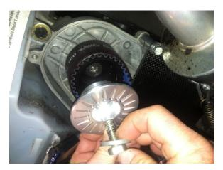
Step 12: Tighten lower driveshaft retainer cap screws to 16 ft/lb.
