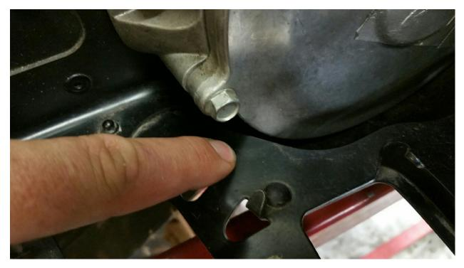
On T3 models this portion of the running boards needs to be trimmed or bent.
