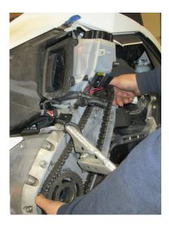
**<u>Step 7</u>**: Locate the new lower pulley retainer from the kit (photo below). Back the 2 pre-installed <sup>1</sup>/<sub>4</sub> - 20 bolts out and apply 1 drop of blue Loc-tite to each bolt.
