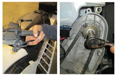
**Step 6:** Remove OEM gears and chain, and jackshaft spacer (top shaft). <u>Thoroughly</u> clean all residual oil from inner chain case face, shafts, etc. using Stoddard solvent, brake cleaner, etc.
