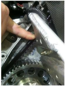
Step 15: Form the composite belt guard around the lip of the OEM chain case lip.
